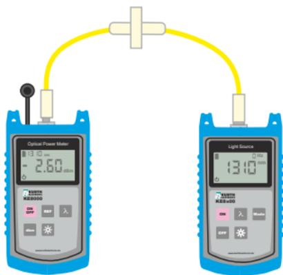
Now disconnect the measuring cable from the power meter and connect the open end via a coupling, e.g. to the fibre section to be measured. The other end of the fibre path is now connected to the level meter. Make sure that the connection at the power level transmitter is not detached or altered.
