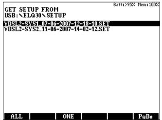
To copy only one of the parameter sets to USB stick draw the highlight to the wanted name and press the **ONE (F3)** key
