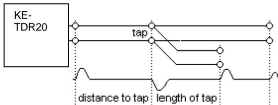
The troubleshooting may be difficult if the tested pair is tapped at many points. In this case, the test should be progressively done with moving from tap to tap.
