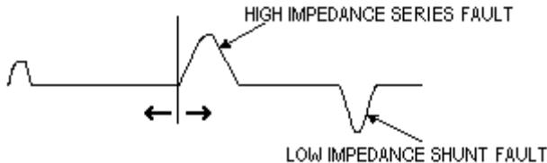
The displayed value of the cursor shows the distance to fault. Remember to deduct the length of the test leads.
