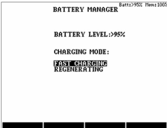
The wanted charging mode can then be selected, and started by using the appropriate keys.
